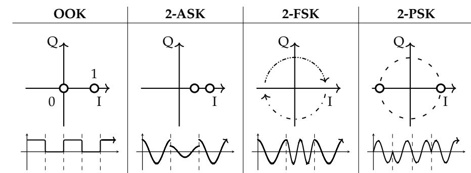
Format names are vague and overlap, the waveform is best understood through the carrier and the constellation chart. Generally the more nodes the more data throughput but with higher loss.
