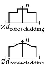
$$\text{Step-Index Delay } \sigma_s \approx \frac{Ln_1\Delta}{2\sqrt{3}c}$$
